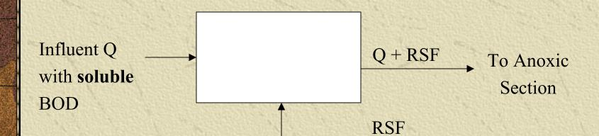
Return sludge with facultative fermentation bacteria and obligate aerobic polyphosphate bacteria or phosphate accumulating organisms (PAOs)
