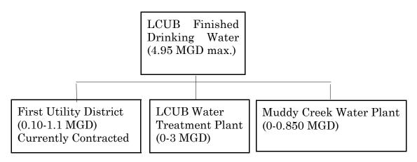
As is outlined in the chart above, LCUB's finished drinking water (4.95 MGD max) is comprised of water produced at LCUB's Nelson Street Water Treatment Plant (3 MGD max) and Muddy Creek Water Treatment Plant (0.850 MGD max) in addition to water purchased from First Utility District (1.1 MGD max under current contract). The water produced at LCUB's Nelson Street Plant comes from the Tennessee River. The water produced at LCUB's Muddy Creek Water Plant comes from the Allen Fine Spring.
