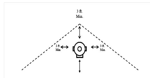
Must be unobstructed within the dashed line triangle area to the roadway.
